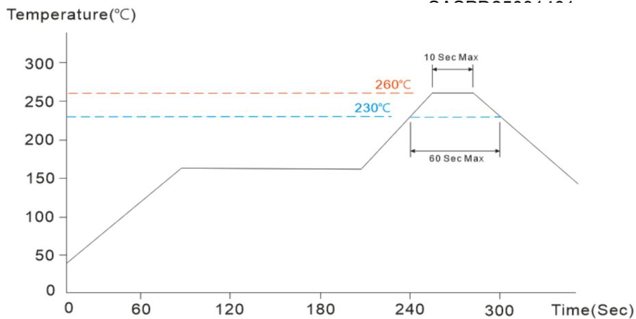
No mechanical and electrical defects are found after testing based on the above profile and keeping under the conditions of room temperature and humidity for 2 hours.
